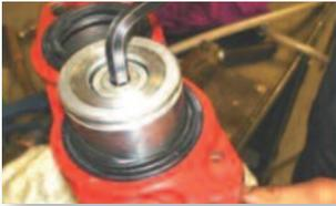
**ROADLINK Rebuilds** each caliper assembly carefully and professionally in a clean environment, using new pistons, seals, boots, bleed nipples and slide pins - every time.
