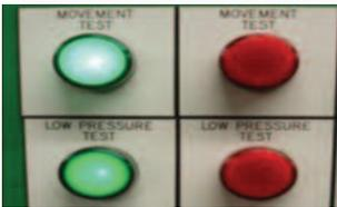
**ROADLINK Tests** every caliper after reassembly on a specially developed test bench, which simulates actual brake application. In the unlikely event of a caliper not being to specification, it is completely re-processed.
